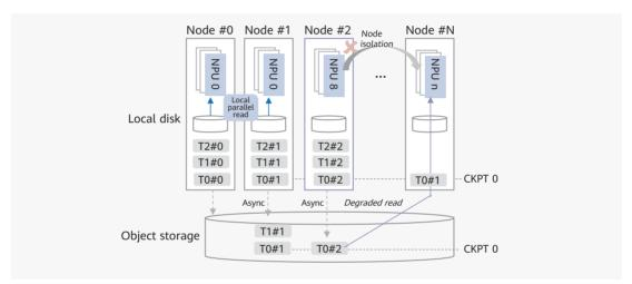
Figure 16: An invalid training epoch due to node faults
