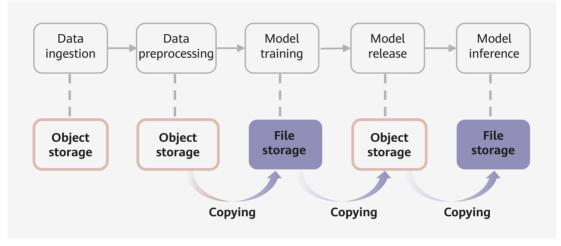
Figure 20: Multiple data copies due to varying protocols
