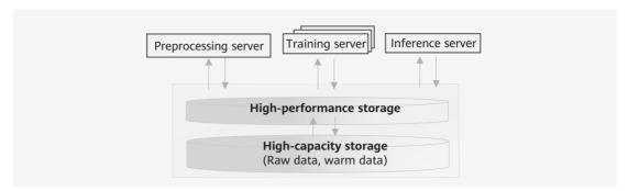
Figure 17: Decoupled storage-compute architecture for on-demand evolution
