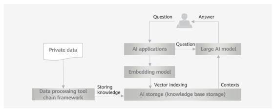
Figure 27: Working process of the RAG knowledge base
