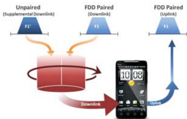
Figure 2: SDL for additional downlink capacity and traffic asymmetry (Source: Qualcomm)
